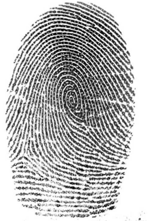
The fingerprint obtained with the FS88H is of such high quality that even the pores located on the finger ridges can be appreciated.
